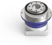
02: The NTP has torsional backlash of  $\leq 5$  arcmin and is now available in four different sizes from 015 to 045, with maximum torques from 56 to 800 Nm and gear ratios from 4 to 100.
